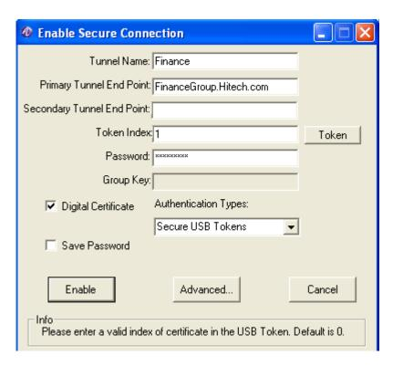
When you enable a tunnel, you can use the **Token** button on the Enable Secure Connection dialog to select a digital certificate in the USB Token.
