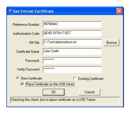
If the Place Certificate in USB Token Check box is checked, Alcatel-Lucent IPSec Client will place the enrolled digital certificate in your USB Token.
